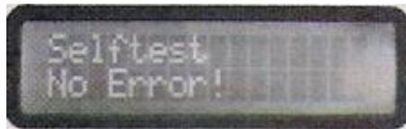
**Figure 5-8: Display After Successful Selftest**
