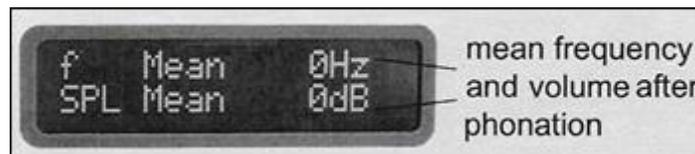
**Figure 5-2: Mean Frequency/Volume Display After Procedure**
